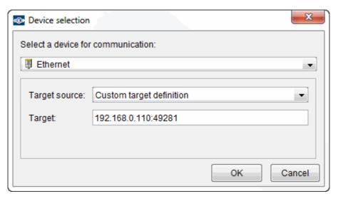
The Ethernet connection can be configured by IP address or host name with an additional port definition.
