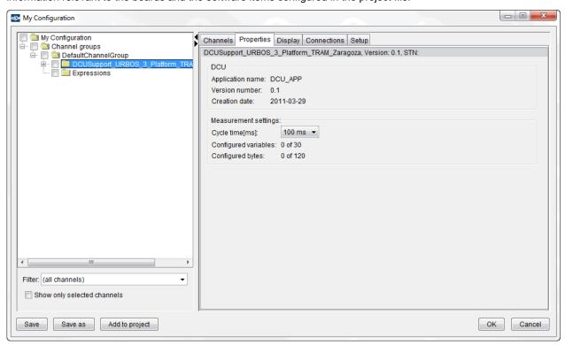
There is information available about the number of configured channels and their size; additionally the cycle time can be configured according to the type of the project.
