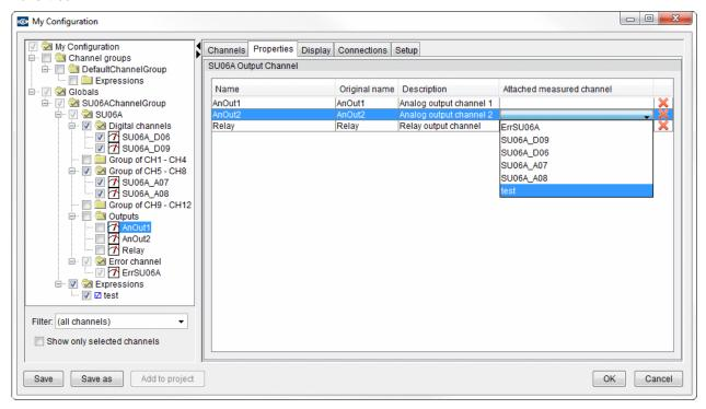
The **Attached measured channel** field can contain expressions or measured channels for controlling output channels (analog and relay) depending on values of running measurement. The result of expressions for analog outputs should be between 0 and 10 V (if the result value is greater than 10, it will be rounded down to 10), whereas the result for relay should be logical (TRUE or FALSE, 0 or 1 etc.).
