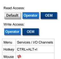
This function allows access to the I/O signals of the boards of the control system. The user can monitor the values of all the inputs and outputs for each board. The user also has the option to force certain output signal values. The display is periodically updated.
