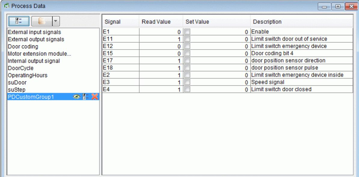
The screenshot shows a window titled "Process Data" with a table of signals. The table has four columns: Signal, Read Value, Set Value, and Description. The "Set Value" column contains checkboxes. The "Read Value" column contains numerical values. The "Description" column contains text descriptions of the signals.
