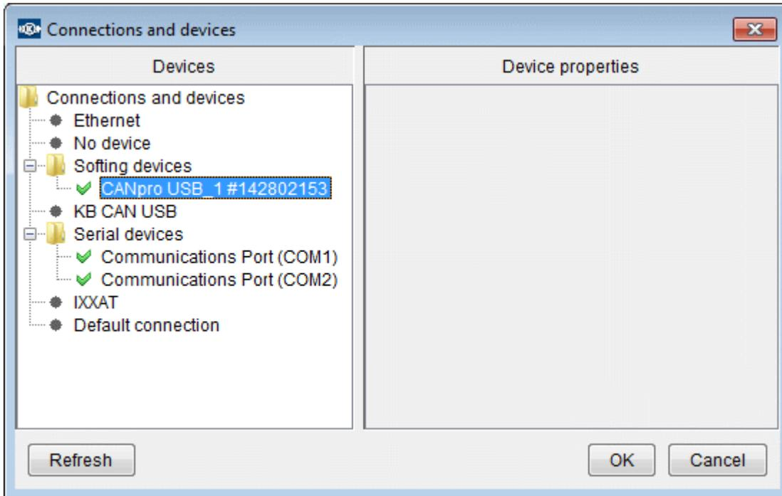
"Default connection" is a special "device"; it refers to the device actually set as ST03A connection.
