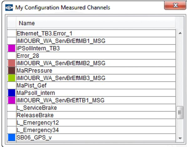
Measured Channels window lists all the channels that are selected for measurement. Only the colour and name of the channels is listed.
