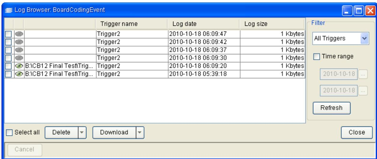
In the table you can find all the logs that have been recorded with the selected configuration. The applicable functionality depends on where the logs are present.
