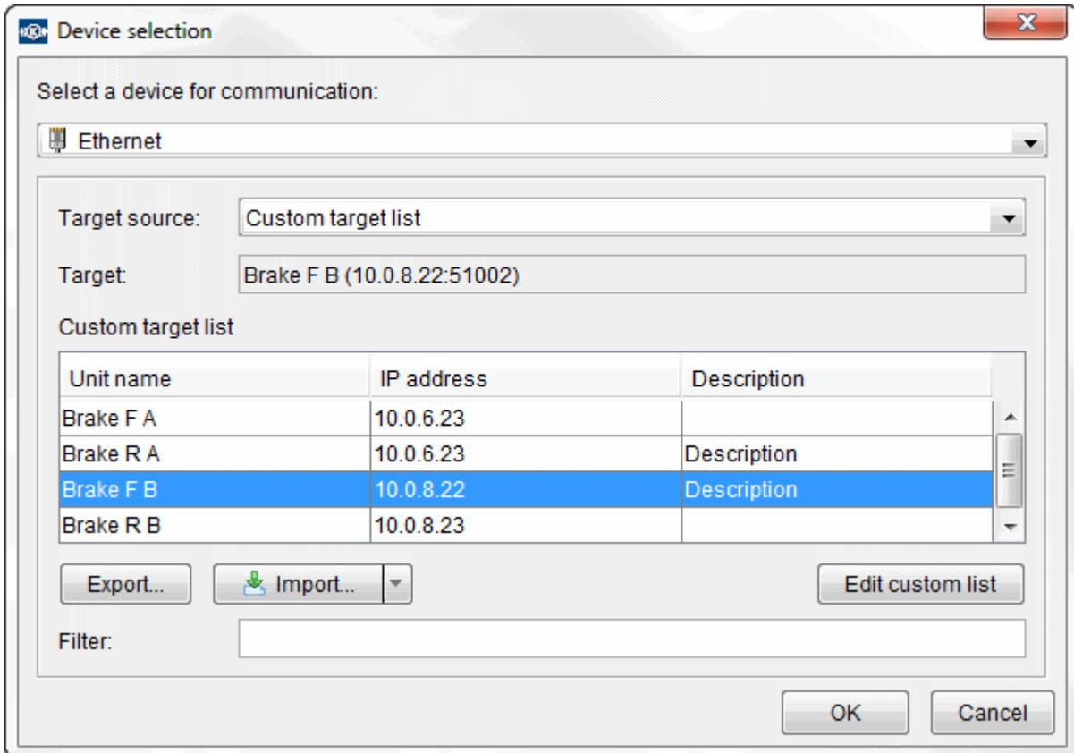
In this case the target to be connected can be selected from a list. The target definitions are stored in a local ST03A version independent file, which means a new ST03A will be able to use your already defined targets.
