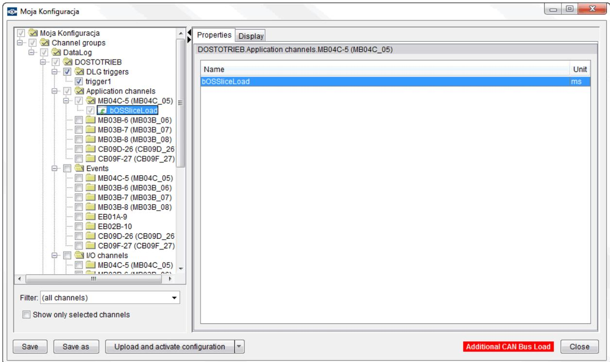
The user can modify or delete application channels on this panel. The name, transformation (factor, offset) and unit columns are editable. All other properties are defined in the project.
