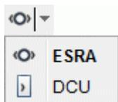
The opened project defines automatically the operating mode (ESRA/DCU). Without project the operating mode is selectable, you can choose ESRA or DCU mode from the toolbar. The [System Mode Icon](#) in the bottom right corner of the main window shows the current mode of ST03A. When a project file is open the project file type (DCU)/(ESRA) is displayed in the title row too.
