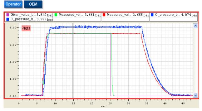
Each graphic plot contains a list of channels (top) and a graphic area. The graphic area contains the channels and the two axes. If the curves are moved so that they have different Y axes the one visible Y axis belongs to the channel that is highlighted in bold.
