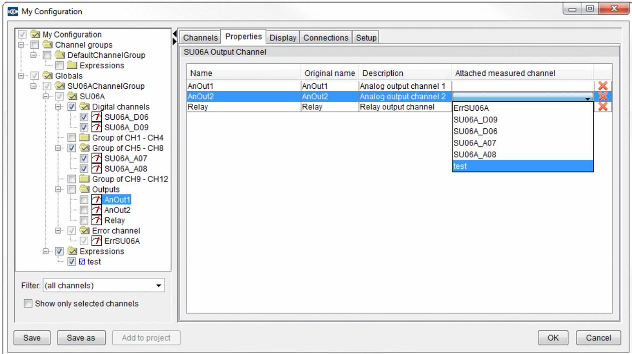
The **Attached measured channel** field can contain expressions or measured channels for controlling output channels (analog and relay) depending on values of running measurement. The result of expressions for analog outputs should be between 0 and 10 V (if the result value is greater than 10, it will be rounded down to 10), whereas the result for relay should be logical (TRUE or FALSE, 0 or 1 etc.).
