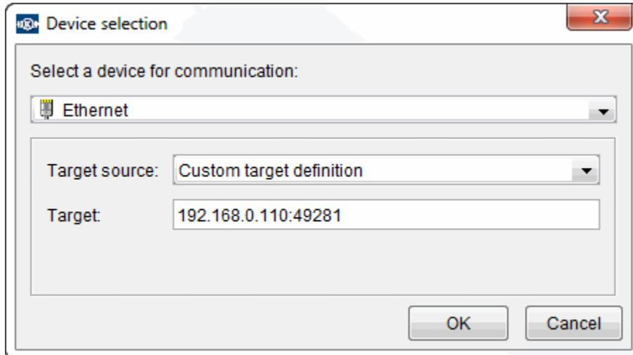
The Ethernet connection can be configured by IP address or host name with an additional port definition.
